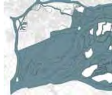
scenario of millenium flood, high watermark at 5.0m NAP
